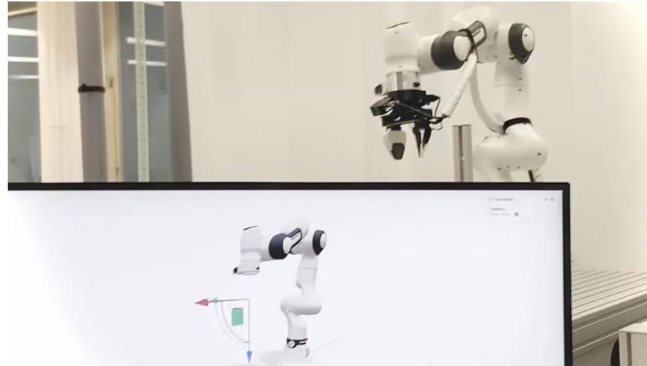
Compliant Robot control
